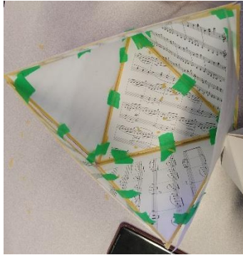
Figure 3. This is the second iteration of the prototype using the paper and spaghetti to simulate wood and plastic.
